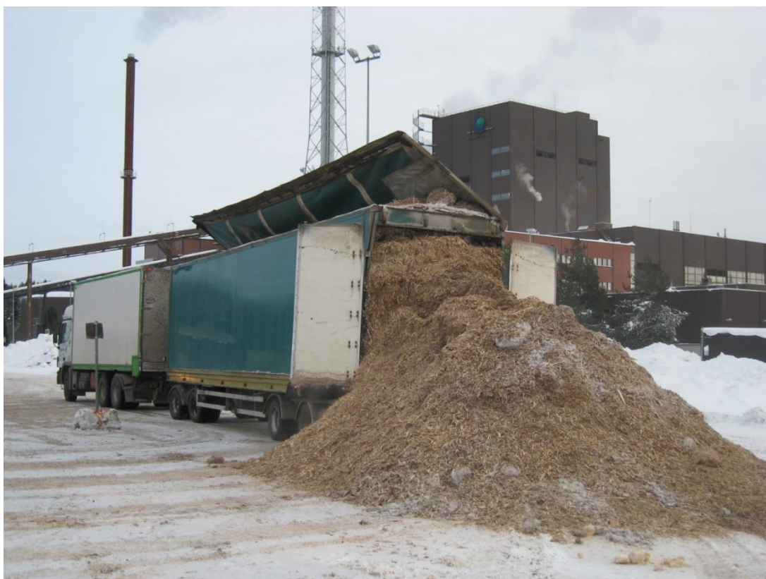
Figure 6. Unloading of willow chips from the truck trailer at Fortum's power plant.
