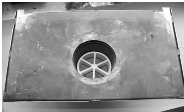
Figure 9: Photograph of the stainless steel tube containing an uncoated monolith directly under the grate
