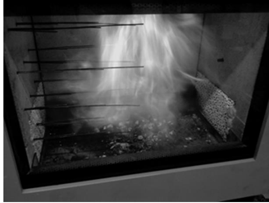
Figure 5: A photograph of the experimental setup with Al 2 O 3 -foams in the lower chamber
