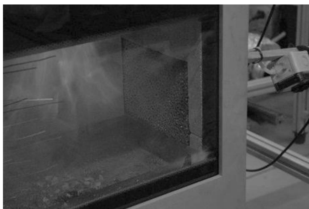
Figure 7: A photograph of experimental setup with bigger Al_2O_3 -foams (size: 140 \times 200 \times 20 \text{ mm}^3 )
