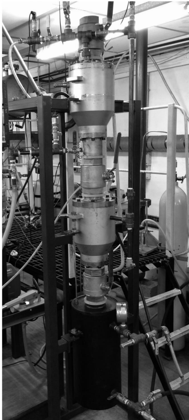
Figure 1. Schematic diagram of the Hydraulic Lock Hopper and the experimental rig.
