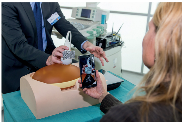
Fig. 1: An unborn infant can be observed in the womb via an ultrasound device, smartphone and BabyAR; a pregnant woman is simulated here with the aid of a ultrasound phantom.
