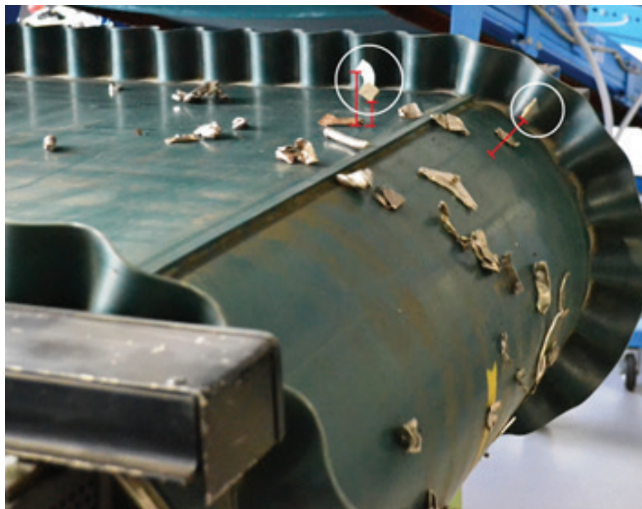
Fig. 1: Separating rare earth magnets with eddy current separators While permanent magnets are ejected using opposing magnetic fields, iron particles are attracted due to their magnetic properties and removed from the field by conveyors.
